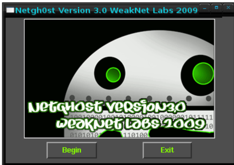
figure 0: The splash start for Netgh0st version 3.0 (the white border is the "Canvas()" function you see in the above code. If your image displays only partially, or too small in the white border you can change it's size with '-width=>"n", -height=>"n"' parameters in the Canvas() function.
